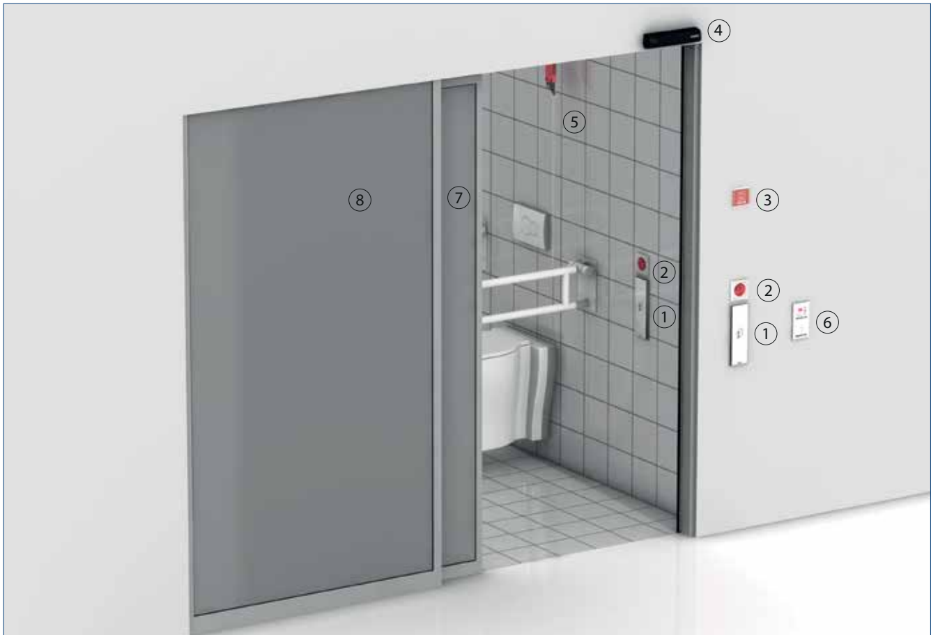
1 = Elbow switch (interior and exterior) | 2 = "Occupied" indicator light | 3 = Emergency off switch (recommended installation height: 1600 mm) | 4 = Active infrared detector | 5 = Emergency call pull switch | 6 = Programme switch with key switch | 7 = Sliding panel ISO-/ toughened safety glass fine-framed with satin-finished film on site, alternatively wooden leaf | 8 = Side panel
